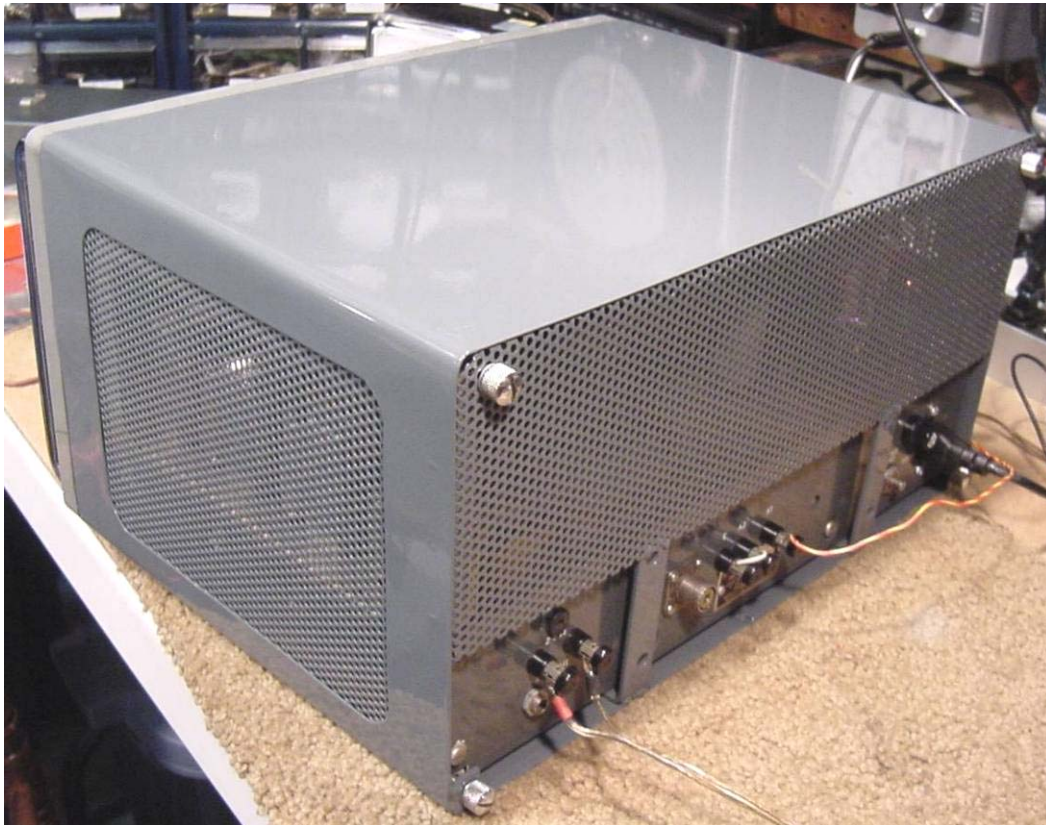
Above/below: rear views of the case with and without the chassis fitted. The colour is called 'Iron Grey' and is the darkest the powder coat shop stocked (it is perhaps a tad on the light side for the purist but looks fine and contrasts ok with the front panel colour).
